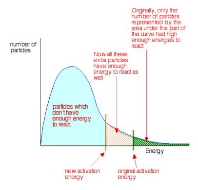
Adding a catalyst has this effect on activation energy. A catalyst provides an alternative route for the reaction with a lower activation energy. This is illustrated on the following energy profile:
